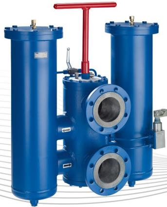
Duplex filters are used in hydraulic systems for separating solid materials from the hydraulic fluids and lubricating oils. They are intended for installation into piping. The filter element can be changed without any operational interruption.
