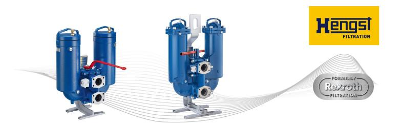
Duplex filters are used in hydraulic systems for separating solid materials from the hydraulic fluids and lubricating oils. They are intended for installation into piping. The filter element can be changed without any operational interruption.
