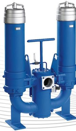
Duplex filters are used in hydraulic systems for separating solid materials from the hydraulic fluids and lubricating oils. They are intended for installation into piping. The filter element can be changed without any operational interruption.
