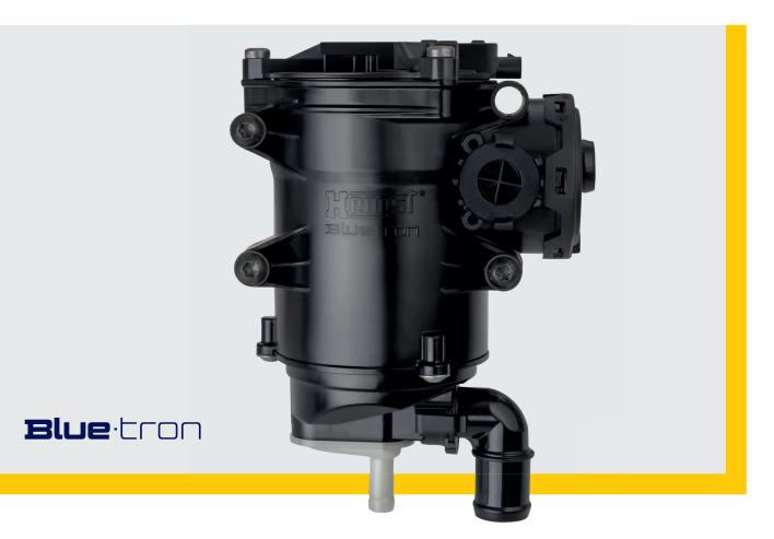
Hengst developed **active ventilation** as part of an overall filter concept for hydrogen engines that also features an electrically driven Blue.tron disk sep**arator**. The latter reliably separates the finest of oil particles from the blowby flow. The cleaned liquid is conducted back to the oil circuit while the gas flows into the intake system via a **pressure regulating** valve.
