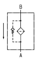
Filter symbol with reverse flow check valve
