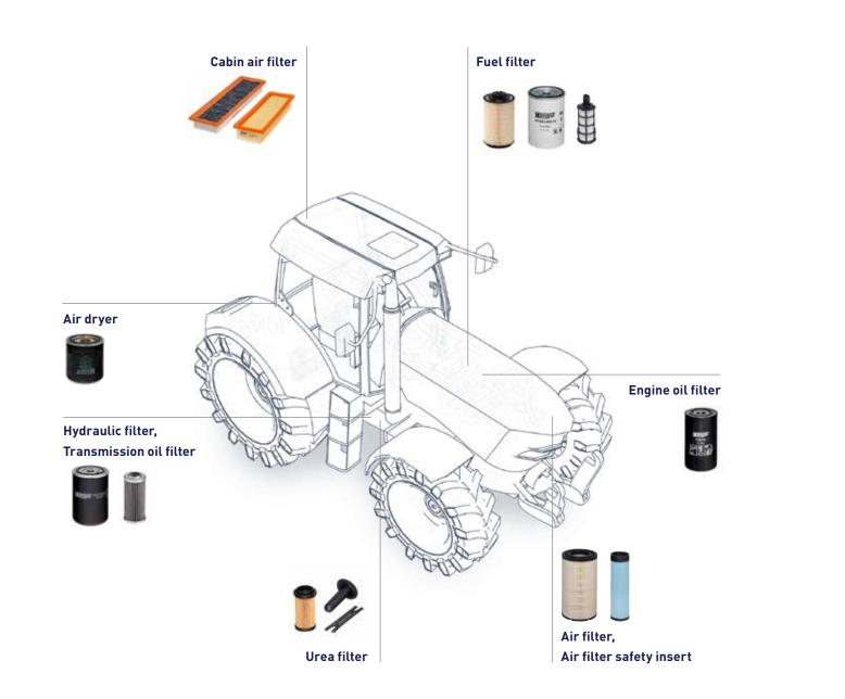
external influences as sand and dust or from wear caused inside the system and help the vehicle operate at peak performance. Hengst offers filtration solutions across all performance classes and emission standards thanks to a constantly growing product portfolio for agricultural and construction machinery.
