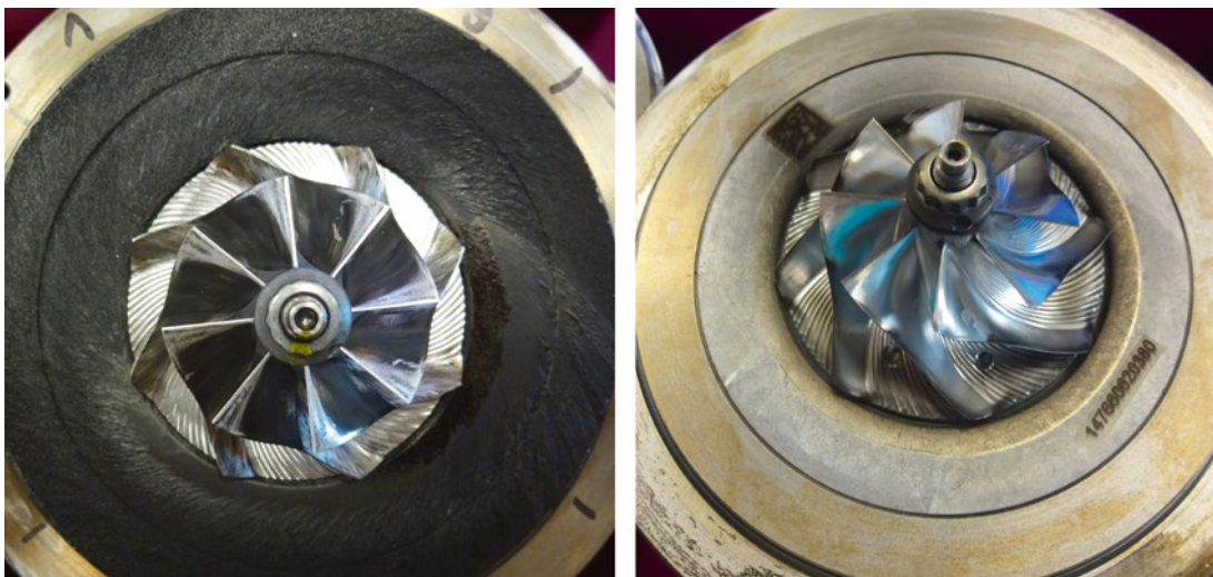
FIGURE 5 Compressor after an endurance run leaving deposits with a passive separator (left) and an electric disc separator (right) (© Hengst)
